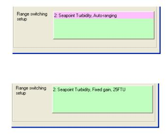
Although readings are taken with different front-end amplifier gains, the data are stored in the logger referenced to the maximum full-scale range. Hence all turbidity readings are referenced to 2500FTU. This means that the calibration
