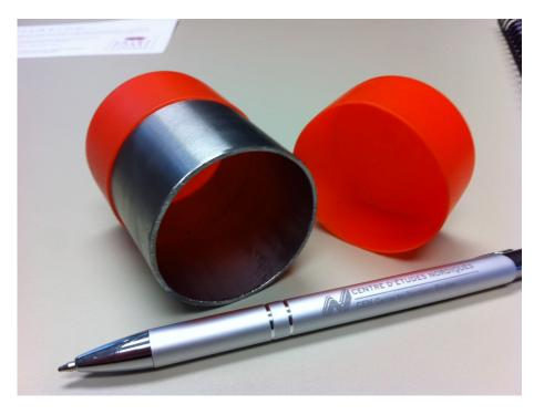
*Figure 1. ADAPT soil sampler used for bulk density determination.*
